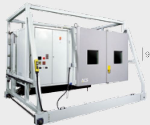
Vibration chamber (capacity 6000 lt approx.) to simulate combined stress (temperature, humidity, vertical and horizontal vibration) on vehicle devices
